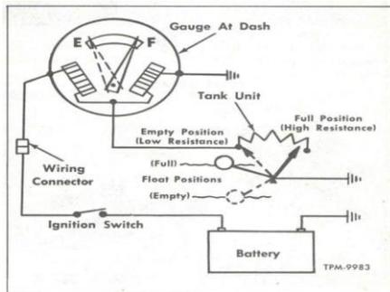
Figure 1—Fuel Gauge Schematic Wiring Diagram
